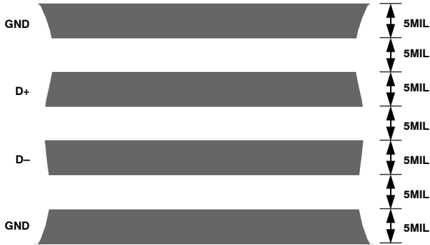
Figure 16. Typical Arrangement of Signal Tracks
